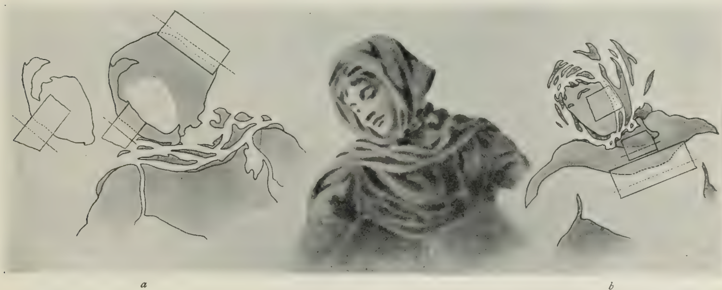
FIG. 6—TINT SHUTTERS, SIMPLE AND COMPOUND, ATTACHED TO STENCIL PLATES FOR THE PURPOSE OF SCREENING PARTS FROM SURROUNDING TINTS
